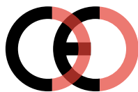
False CE Mark (too close)
